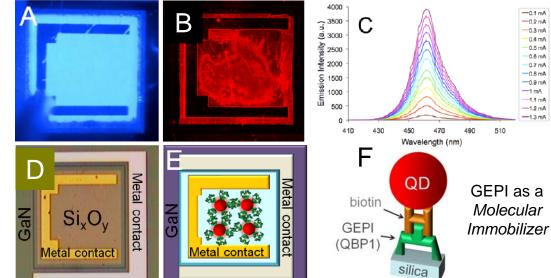
(A) DF Image, (B) Electroluminescence, and (C) Profiles at 462 nm at various levels of driving current at room temperature. (D) Plan view of the fabricated LED device with microarchitectured metal, semiconductor, and dielectric regions (light optical microscopy) and (E) its schematics, the showing (QBP1-bio)/(SA-QDot) hybrid construct targeted assembled only on the silica regions of the device. (F) The GEPI construct.
