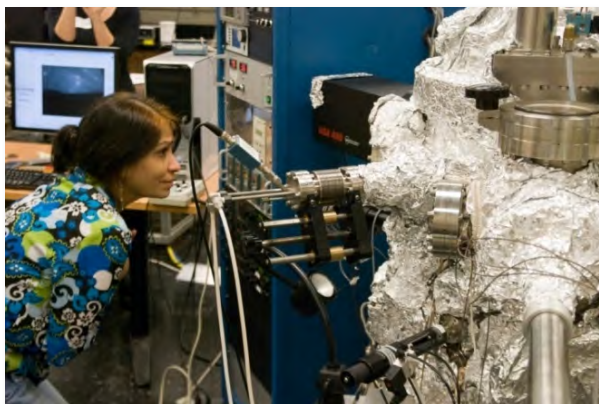
Nanofabrication: MBE with Fred Walker
