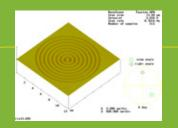
**Optical bulls-eye structure:** Nanoscale and microscale structures fabricated in metals will be used to manipulate the propagation properties of light.
