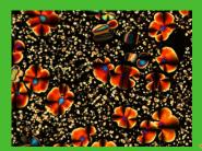
Complementary nanoDNA stacks end-to-end in water to form rod-shaped aggregates that in turn make liquid crystal phases.
