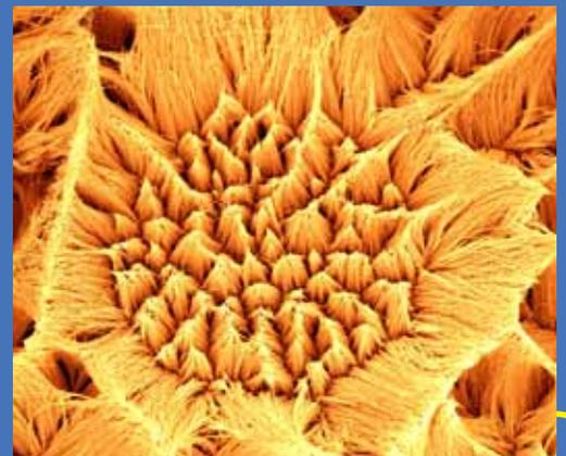
Nanorods of 15 nanometers in diameter and 10 microns in height made of high surface area metallic glasses for catalysis
