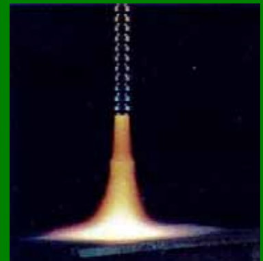
Jet plume from a plasma spray torch.
