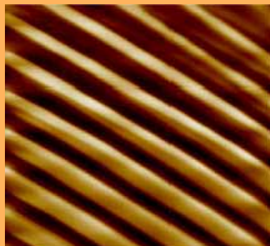
20 nm-high Co wires, directly transferred onto a dendrimer-modified silicon substrate by a patterned stamp.
