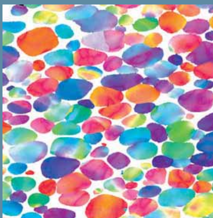
Granular microstructure: the colors correspond to the local orientations of tungsten crystals.
