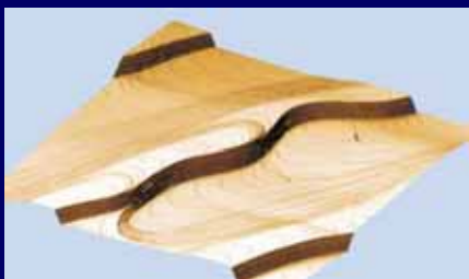
STM image of single-atom steps - a complex non- equilibrium structure - created by an external electric field.
