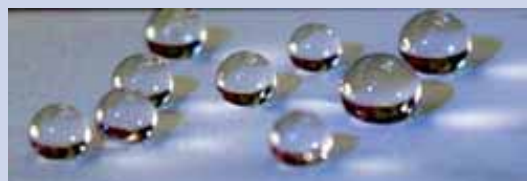
Water droplets on a super-hydrophobic surface mimic the water-repellence of the lotus leaf.
