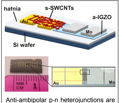
Anti-ambipolar p-n heterojunctions are fabricated at the wafer-scale using s-SWCNTs and a-IGZO.
