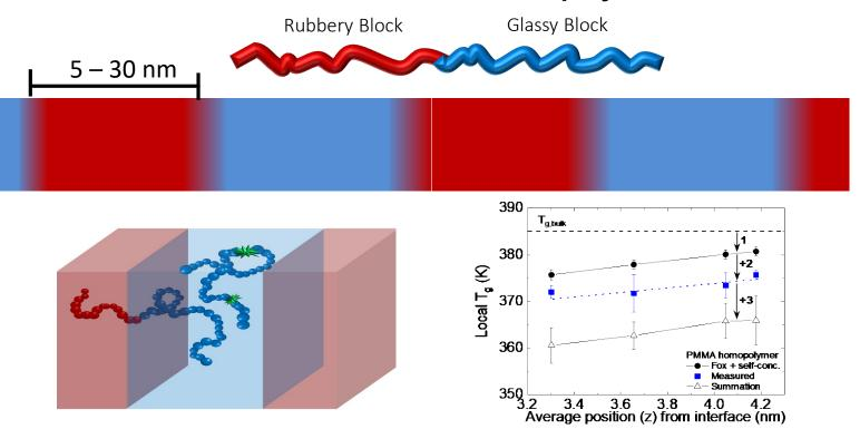
**IRG-2** members developed an approach to directly measure the influence of chain connectivity on the glass transition temperature of copolymers for the first time. This development is important as it provides insights into the design of copolymer interfaces for applications in which transport of entities is important.
